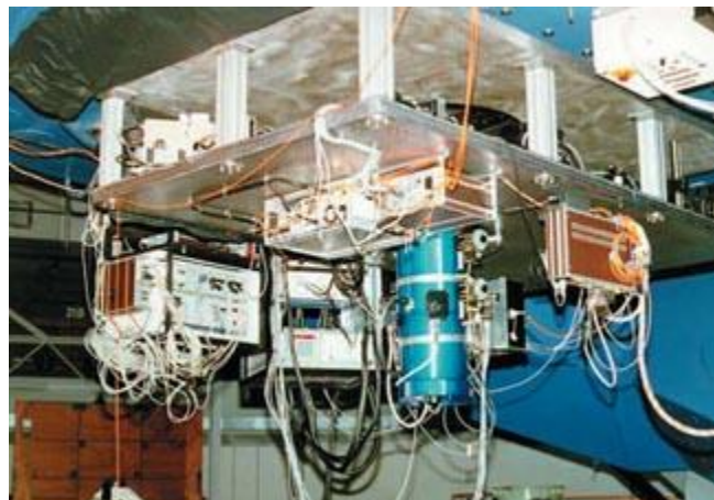
Figure 7. The ALFA adaptive optics system installed on the Max Planck Institute for Astronomy's telescope in Calar-Alto, Spain.
